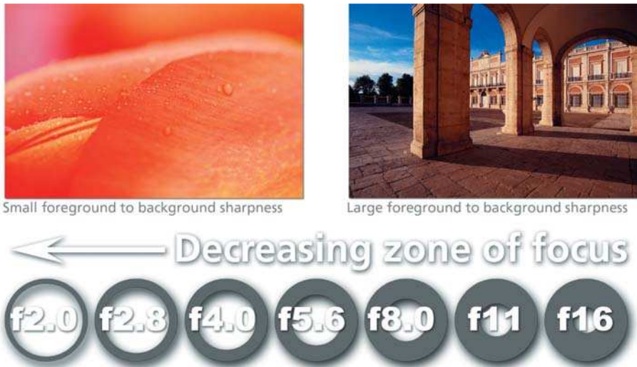
Figure 8.5 The aperture setting also controls the depth of sharpness in the picture. Smaller holes are used to create pictures where sharpness extends further into the image. Large apertures tend to restrict sharpness to just the subject that is focused.
